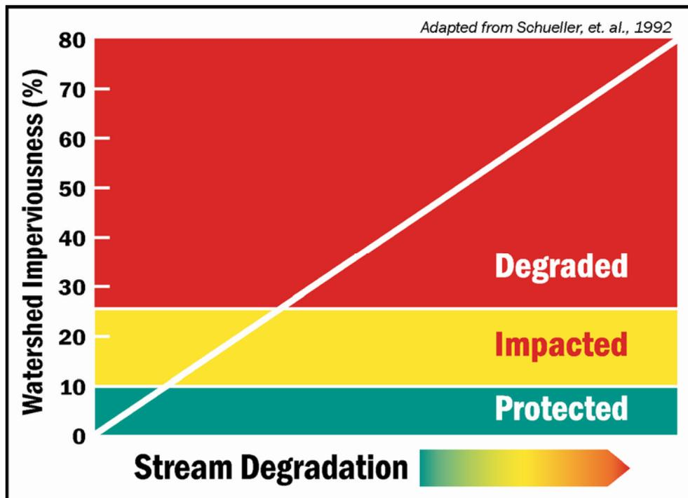
Figure 3. Stylized relationship between watershed imperviousness and receiving stream impacts.
